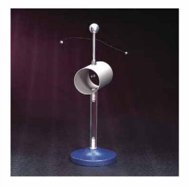
This is a very noticeable air movement which can easily be shown by holding a candle flame near the dome. This air movement is often called the electric wind. When the Van de Graaff Generator is turned off, the dome voltage immediately subsides and the wind stops. As long as the electric wind is blowing it interferes with charging of the pith balls.
