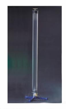
FOUNTAIN IN A VACUUM: The tube with its stoppers in place is mounted on the tripod. The tube is exhausted by connection to the vacuum system. The valve is closed and the connection to the vacuum system is removed and replac-ed with a short length (2-3 ft) of rubber tube. The free end of the hose is then placed under the surface of a water supply and the valve opened. Water is forced into the cylinder by outside air pressure in a powerful jet which rapidly fills the cylinder.
