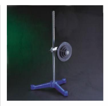
If you want to work with actual pulley diameters, wrap a piece of string around the pulley and put a pencil mark across any two adjacent turns. Measure the length between marks and divide by pi.
