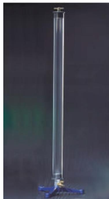
**FOUNTAIN IN A VACUUM:** The tube with its stoppers in place is mounted on the tripod. The tube is exhausted by connection to the vacuum system. The valve is closed and the connection to the vacuum system is removed and replaced with a short length (2-3 ft) of rubber tube. The free end of the hose is then placed under the surface of a water supply and the valve opened. Water is forced into the cylinder by outside air pressure in a powerful jet which rapidly fills the cylinder.
